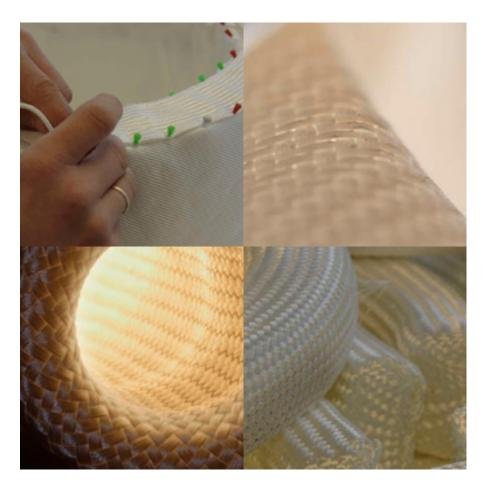
ALF is available as woven cloth, braided sleeve, tape, rope, yarn and sewing yarn and is appropriate for countless applications including the following:
